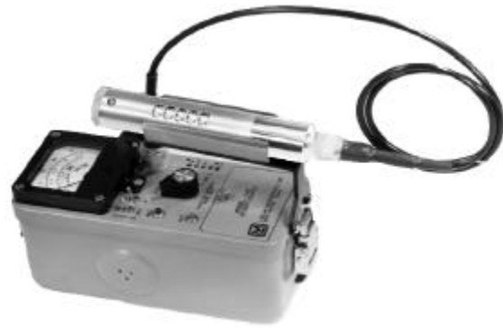
Figure 2-6. Geiger-Mueller Counter with an Energy-compensated Gamma Probe. (Photo courtesy of Ludlum Measurements, Inc.)
